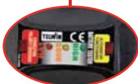
EN | With tester and protection. Indicates charge status, inverted polarity and active alternator.
