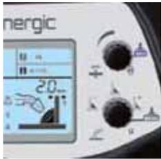
Set the material thickness and start welding!
